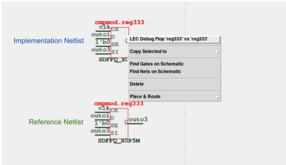
Figure 44: Debug non-equivalence by counter-example back-annotated
